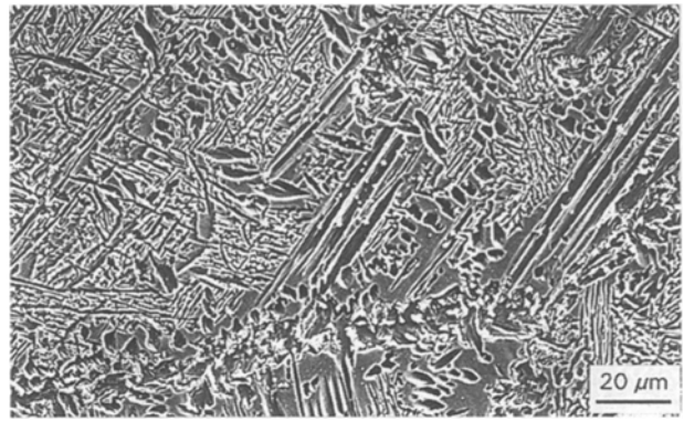
Figure 7 Microstructure of the sample aged at 500 °C for 5 min.
