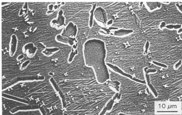
Figure 5 Equilibrium \alpha + \gamma phase in a martensitic matrix for the sample aged at 400 °C for 12 h.
